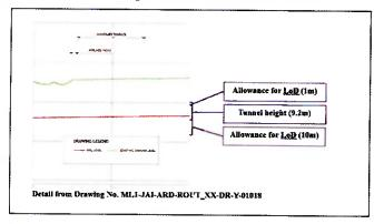
Therefore the land that will be **authorised** to be acquired under the Railway Order for the purpose of a tunnel is in the shape of a continuous tube with a rectangular face, 30m in width and 20.2m in height. This is the complete answer to the second issue raised.
